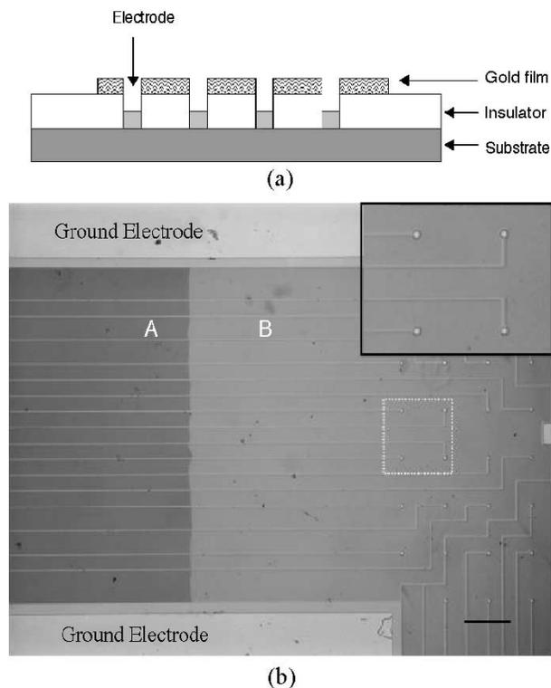
Fig. 1. Gold-coated MEA. (a) Schematic of partial gold coating on MEA, not to scale. (b) Bright field image ( $5\times$ ) highlighting the original insulator (A) and the gold overlay (B), (inset) microelectrodes, large ground electrodes are seen at top left and bottom left of the picture. Scale bar =  $200 \mu\text{m}$ .
