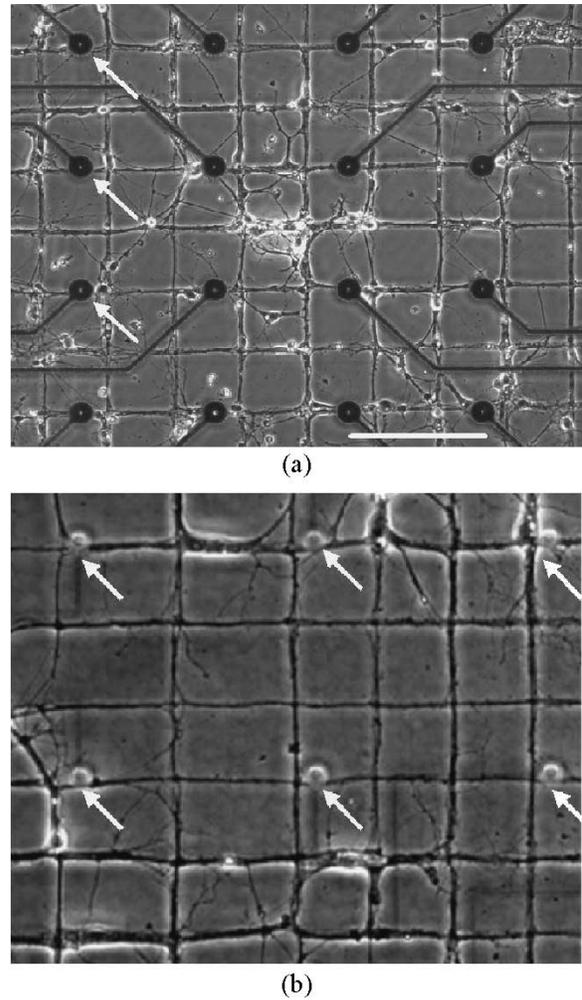
Fig. 5. Neuronal circuit created on gold-coated MEA whose original insulator is  $\text{Si}_3\text{N}_4$  (a) or polyimide (b). Cell growth near electrodes (arrows) was induced by precise alignment of predefined pattern to electrode layout through  $\mu\text{CP}$ . The grid patterns in (a) and (b) have a different spacing. Cell density: 100 cells/ $\text{mm}^2$ . Pictures taken at 12 DIV (a) and 15 DIV (b). Scale bar = 200  $\mu\text{m}$ . From *Proc. 25th IEEE EMBS Annu. Int. Conf.*
