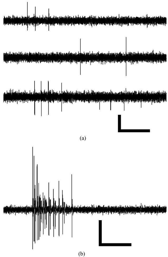
**Fig. 5** Extracellular recordings from a rejuvenated old MEA (14 DIV) (a) and a microstencil attached gold substrate MEA (28 DIV) (b). Scale bar:  $50\ \mu\text{V}$ , 200 ms
