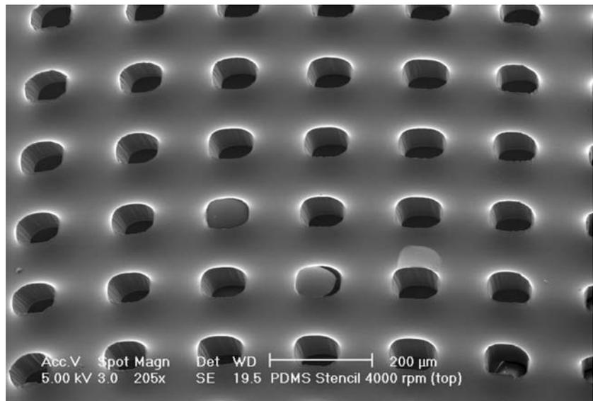
in a thickness of  $41 \mu\text{m} \pm 5 \mu\text{m}$  (mean  $\pm$  SD,  $n = 3$ ). The resulting PDMS microstencils were mechanically durable for repeated attachments and detachments.
