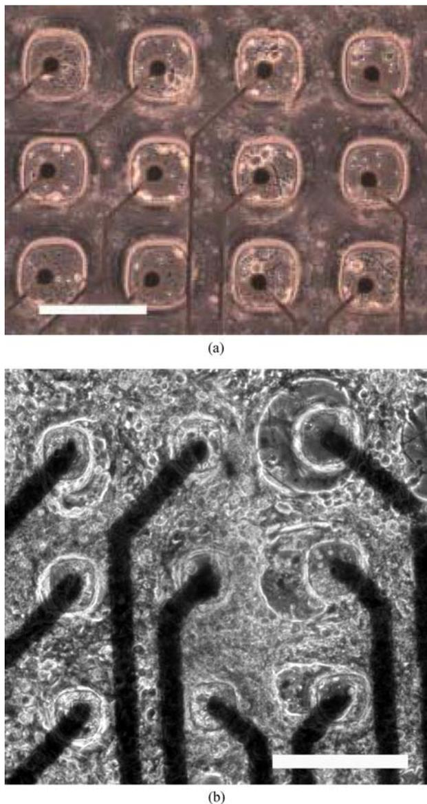
**Fig. 4** Hippocampal neuronal cultures on assembled devices. (a) A microstencil (hole size of  $100\ \mu\text{m}$ ) on top of an old commercial MEA (14 DIV, cell plating density:  $200\ \text{cells}/\text{mm}^2$ ). (b) A microstencil (hole size of  $50\ \mu\text{m}$ ) on a gold pattern substrate on a glass slide (28 DIV, cell plating density:  $1000\ \text{cells}/\text{mm}^2$ ). Scale bar =  $200\ \mu\text{m}$
