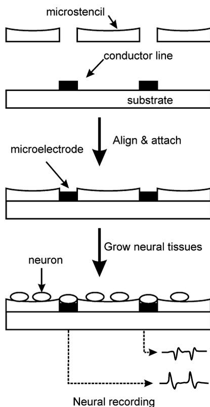
**Fig. 1** Schematic illustration of a single-use MEA
