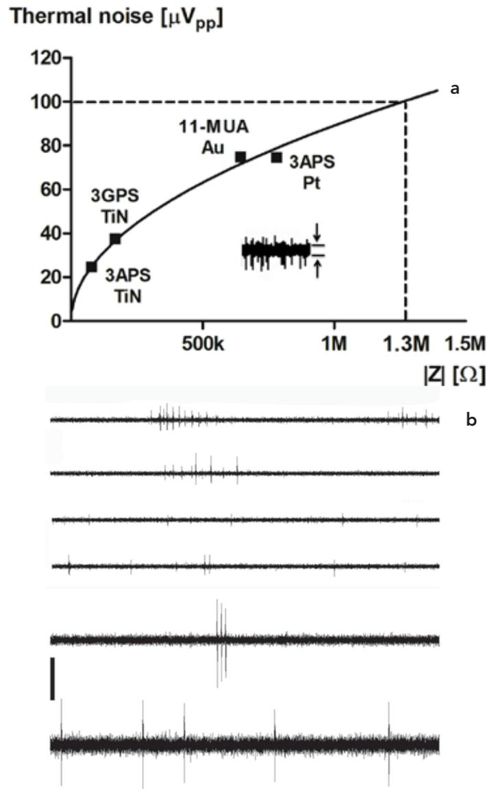
**FIGURE 6.** (a) Theoretical thermal noise peak-to-peak value curve and measured values (square dots) from SAM modified electrodes.  $Z$  value at 1 kHz. (b) Examples of neural recording from 3APS modified platinum black electrodes (top two traces, 33 DIV, SNR 6.5, 8.8), 3APS modified titanium nitride electrodes (middle two traces, 19 DIV, SNR 5.7, 7.5), and 11-MUA modified gold electrodes (bottom two traces, 15 DIV, SNR 18.8, 8.0). Time span: 2 s; scale bar: 100  $\mu V$ .<sup>60</sup>
