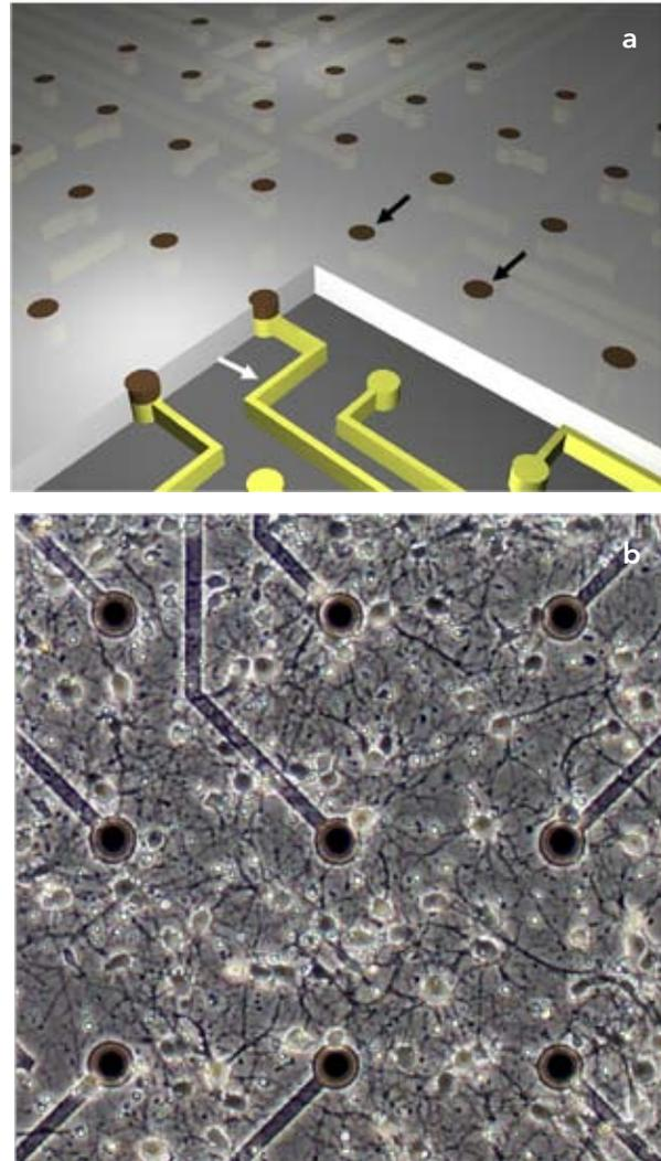
**FIGURE 1.** (a) Planar-type MEA with an array of embedded microelectrodes (black arrows). Conductor lines (white arrow) are insulated by organic or inorganic materials. (b) Dissociated hippocampal neurons are grown on an MEA. Black dots are electrodes and straight lines are conductor lines. Interelectrode spacing: 200  $\mu\text{m}$ .
