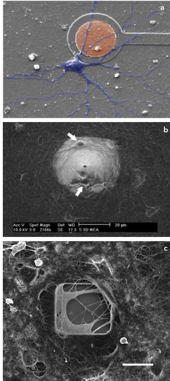
**FIGURE 2.** Neuron-electrode couplings of various MEAs. (a) Flat type MEA, 11 DIV. (b) 3D tip shape MEA, 24 DIV. Arrows indicate attached somata on the electrode. (c) Recessed type MEA, 24 DIV, scale bar 20  $\mu\text{m}$ . Scanning electron micrograph.
