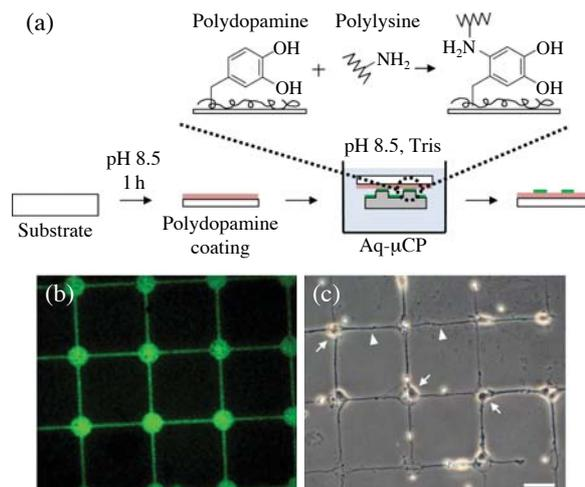
**Figure 4.** (a) The schematic procedure of covalently linking FITC-PLL patterns to polyDAs. (b) FITC-PLL patterning on polyDA-coated glass coverslips at pH 8.5. (c) Hippocampal neurons cultured for 3 DIV (arrows: cell bodies; arrowheads: neurites). The pattern was printed with 20 g of pressure after the sonication for 1 min. Scale bar is 50  $\mu\text{m}$ .
