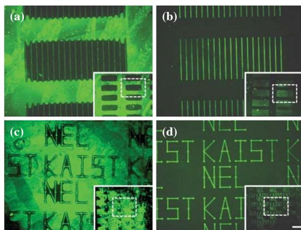
**Figure 2.** Comparison of dry- vs. aq- $\mu$ CP of wide-spacing fine patterns of FITC-PLL. (a, b) Thin line array patterns printed by dry- $\mu$ CP (a) and aq- $\mu$ CP (b). (c, d) KAIST/NEL patterns printed by dry- $\mu$ CP (c) and aq- $\mu$ CP (d). All images are the magnified part of inset images. Each pattern was printed with 20 g of pressure after the sonication for 1 min. Scale bar is 50  $\mu$ m.
