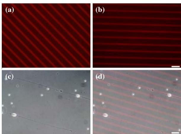
**Figure 3.** Immunolabeled (a) laminin patterns (line width: 5  $\mu\text{m}$ ; spacing: 25  $\mu\text{m}$ ) and (b) fibronectin patterns (line width: 3  $\mu\text{m}$ ; spacing: 30  $\mu\text{m}$ ) printed on glass coverslips. (c) Phase-contrast image of cultured hippocampal neurons on laminin patterns and (d) overlaid with laminin patterns (on-pattern area: red).
